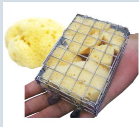
Standard River Sampler Made with Sponge
